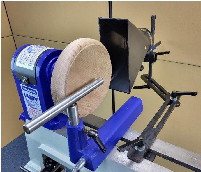
The dust hood can also be used in the vertical position by turning the dust hood arm by 90 degrees.
